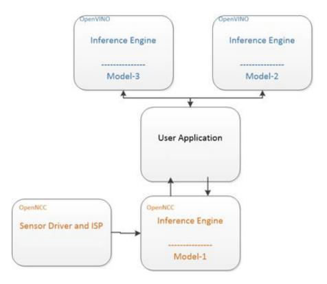
In ncc\_cdk/Samples/Demo/work with OpenVINO demonstrated how to combine OpenNCC and OpenVINO on Host PC to implement a distributed AI system.
